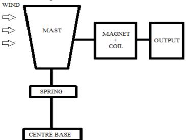
As shown in the block diagram, when wind strike to the mast then according to the vortex principle the mast start oscillating in forward and backward direction. The magnets which are connected to the mast also start oscillating. Due to this oscillation of magnets change in magnetic field produce and flux are cut by the stationary coil conductors according to the faraday's law of electromagnetic induction.
